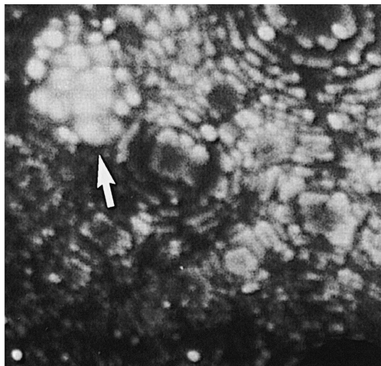
Fig. 2. Field ion micrograph of spherical molybdenum carbides in the weld B surveillance material.
